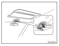
To open the sunroof to the vent position, push the front part of the switch. To return the sunroof to its original position, push the rear part of the switch and hold it until the sunroof reaches the desired position.
